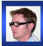
Fig. 1. (left) The Optalert™ system of IR oculography. An LED housed in the bottom of spectacle frames emits pulses of IR light directed up at the eye. The light reflected back from the eye is recorded at 500 Hz by a phototransistor in the frame beside the LED. This gives a measure of the position of the eye and eyelids.
