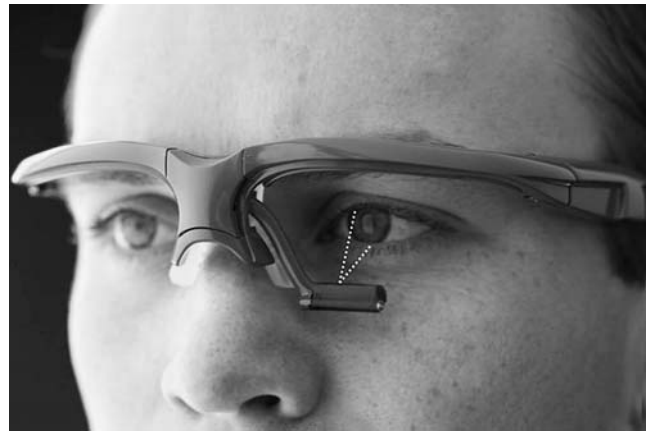
Fig.1 The glasses frame, shown here without lenses, with IR transducers in the arm attached to the frame, and showing the direction of the IR light pulses directed up at the eye
